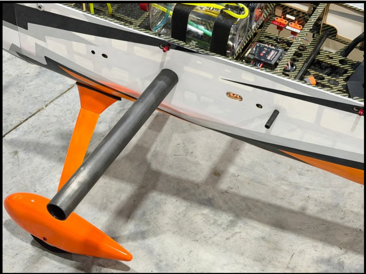
Both the wings and horizontal stabilizers feature a double-tube anti-rotation system.
