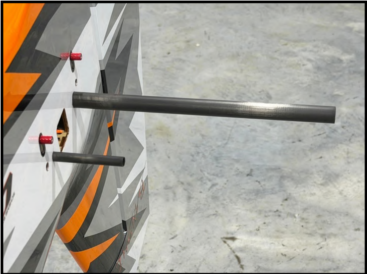
Both the wings and horizontal stabilizers feature a double-tube anti-rotation system.
